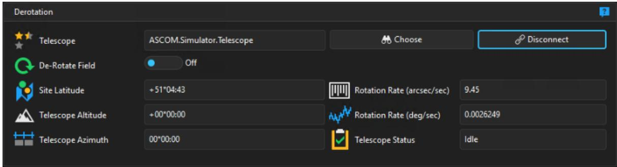
Unity Platform needs connectivity with your ALT-AZ mount via ASCOM Client. It receives your site latitude and longitude along with the celestial target coordinates (target altitude and azimuth). Having this information it continuously updates the parallactic angle and pushes the rate of rotation commands to the Falcon v2 rotator.
