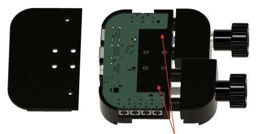
Use a 2mm Allen hex key to untie the set screws that are holding the M8 bolts
