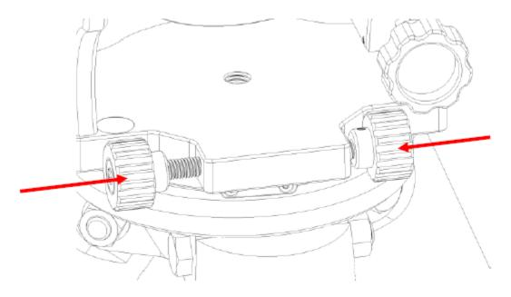
We loosen both Azimuth adjustment knobs.
