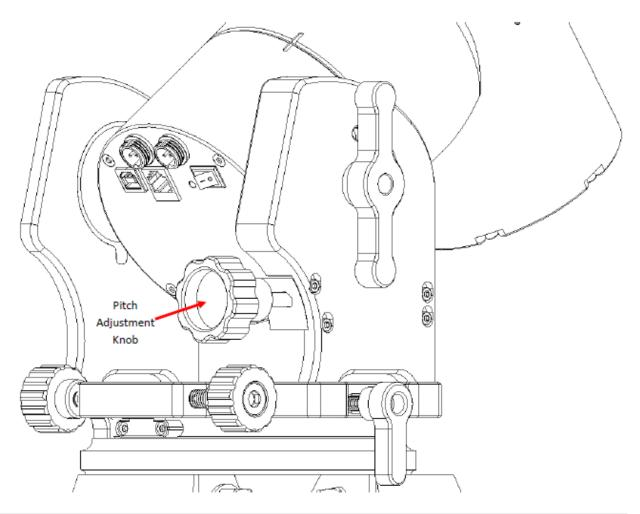
**Important:** The altitude adjustment utilizes a worm gear mechanism so for more accurate results we finish the final adjustment with an **UP** move (counterclockwise) to clear any backlash. Even if we must go down we will go a little further and we will finish with an **UP (counterclockwise)** adjustment.
