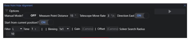
**Measure point distance**: The distance between measure points. If you choose a bigger value, be sure that you don't reach a meridian limit and that any part of your setup doesn't hit the tripod. The plugin uses three points, so if you choose  $15^{\circ}$  the total distance will be  $30^{\circ}$  ( $0^{\circ} - 15^{\circ} - 30^{\circ}$ )
