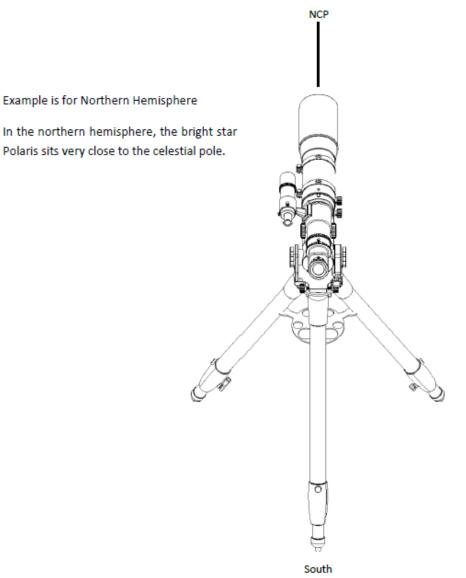
We stand behind the mount and align the whole setup roughly with Polaris. We can use the electronic leveler to adjust mount's angle to match our latitude. To do that we have to loosen the altitude tensioners and fasten them again after completion.
