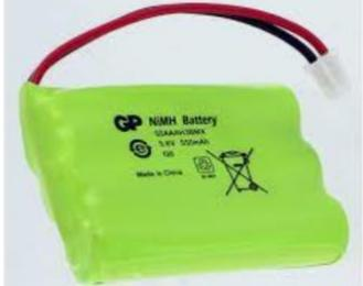
Typically, NiMH batteries can be recharged hundreds of times. However, battery life is limited to up to 5 years. After that, it can be easily replaced with a new rechargeable battery pack. In order to do that:
