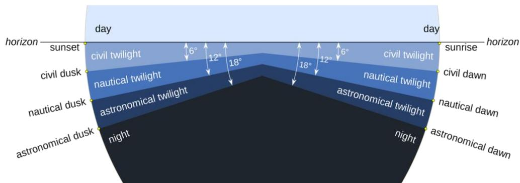
Morning astronomical twilight begins (astronomical dawn) when the geometric center of the sun is 18° below the horizon in the morning and ends when the geometric center of the sun is 12° below the horizon in the morning. Evening astronomical twilight begins when the geometric center of the sun is 12° below the horizon in the evening and ends (astronomical dusk) when the geometric center of the sun is 18° below the horizon in the evening.
