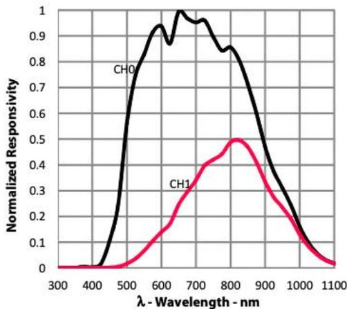
Spectral Responsivity: Two channel response allows for tuneable illuminance (lux) calculation regardless of transmissivity of glass.
