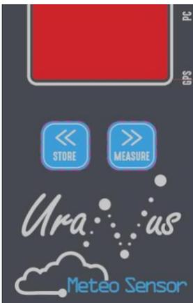
Keep pressing [>>] (**Measure**) button for **2 seconds** to trigger a Sky Quality measurement. Remember to point the device towards the area of the sky you would like to acquire a light measurement.
