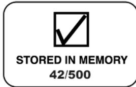
All sensor values are stored into internal memory. Uranus displays a confirmation screen with the memory bank number that was used. In above example Uranus has 42 used out of 500 available records in memory. Press any button to exit this screen.
