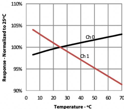
White LED Response vs Temp: Effect of temperature on the device response for a broadband white light source. A temperature compensation algorithm is automatically applied after every readout.
