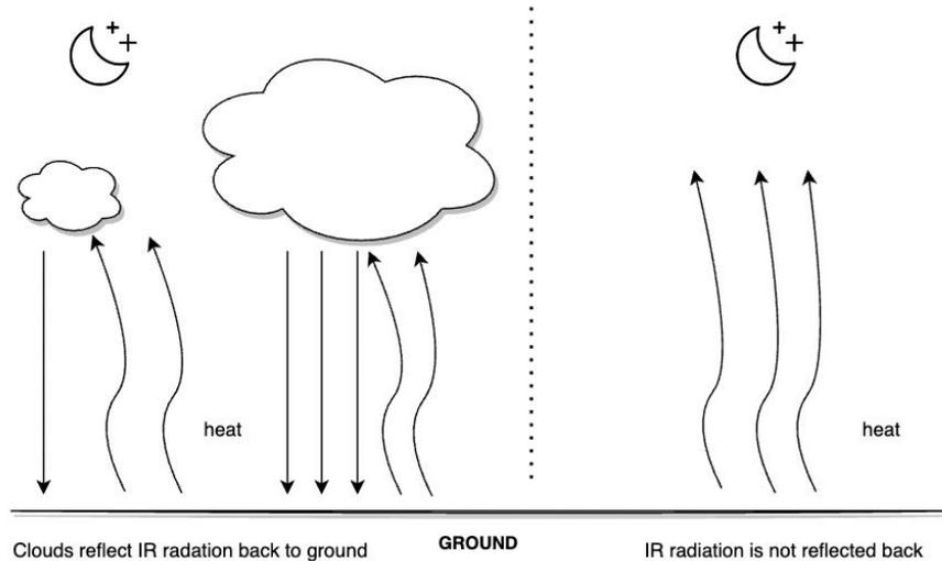
Lots of factors affect the actual sky temperature. Your geographical latitude, the ambient temperature and conditions in troposphere will shift the sky temperature so a correction model is automatically applied by the Uranus device.
