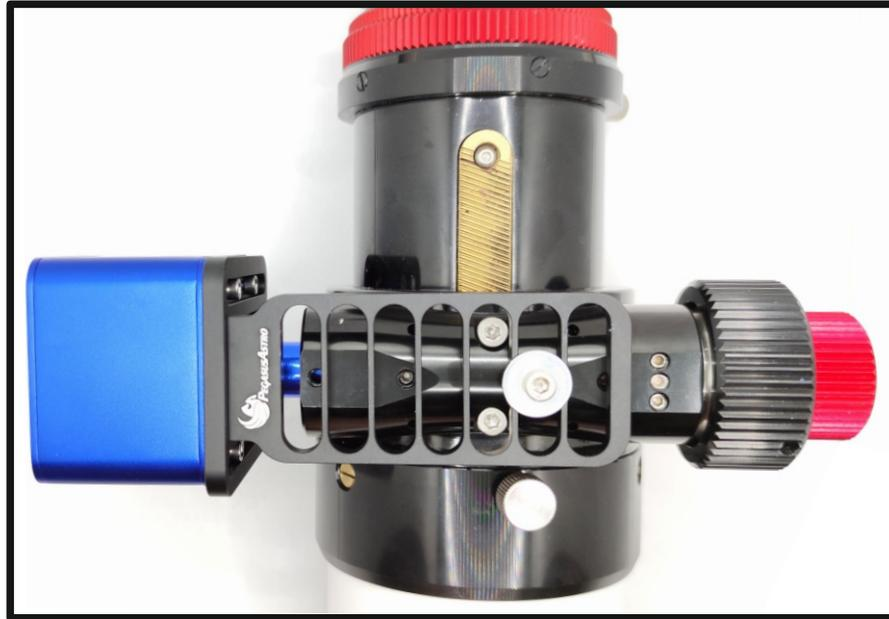
**Adjust the motor up or down to align it with the focuser's shaft**
