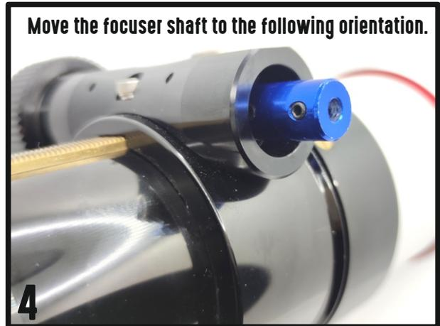
**Attach the motor to the focuser and join the coupler with motor shaft.
