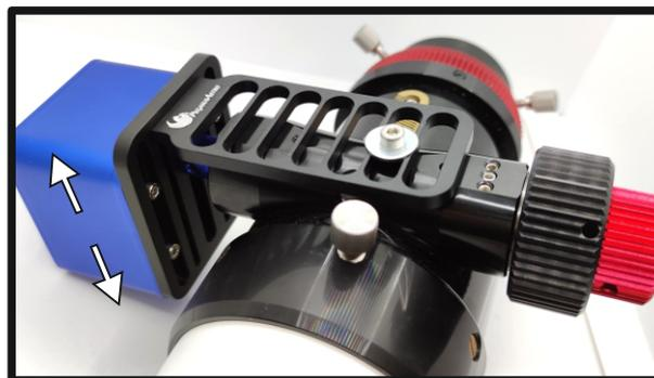
**Use your 2mm Allen key and tight well the set screws on the motor side.**
