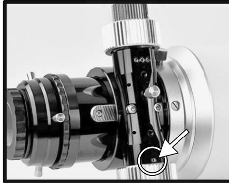
Remove telescope focuser's coarse knob.
