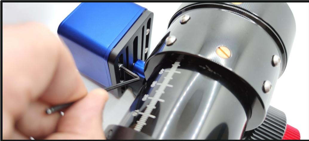
**Once you have installed the motor kit, you don't need the drawtube brake, as the motor locks the shaft.
