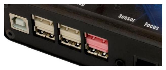
USB2 High Speed Ports can turn ON or OFF via the supplied software. (Please notice: there is no option to selectively switch a port on / off. All ports, except 6<sup>th</sup>, switched ON / OFF **globally**)
