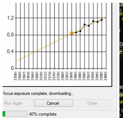
In the end you should see a "V" and a focus point chosen that is very close to both the HFR and focuser position.
