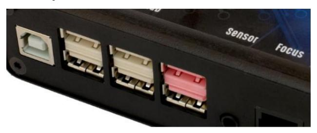
USB2 High Speed Ports can turn ON or OFF via the supplied software.
