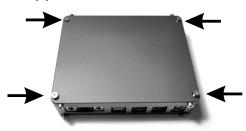
Step 2 Untie the four (4) stock screws from one side of your old enclosure, displayed by the black arrows.
