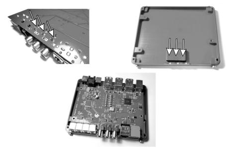
Step 4 Place first the USB HUB side of the top part as shown in the photo below.
