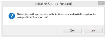
⇒ On yes, the rotator will start moving anticlockwise (reverse) until it senses / reaches the zero limit. When the limit is found, rotator will mark this position as the zero degree point.
