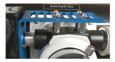
After that you need to remove at least 2 side screws and replace them with longer. Now you can attach the bracket and tight down all the parts together.
