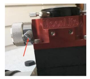
**Step 2:** Match up the focuser shaft thickness with one of the included motor couplers. One side of them is always 5mm (that side goes to the motor shaft). Tighten very well the 2 grub screws on the focuser side.
