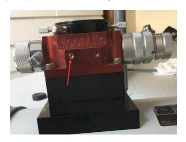
**Step 4:** Tighten all the grub screws of the motor coupler and the 4 silver alen bolts that hold the motor to the bracket.
